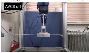
Active vibration control system (AVCS) for smallscaled compound helicopter model
